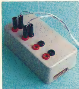
The Box This is the finished box, showing the minicon plug and input/output leads. Care must be taken in cutting the board and the slot in the box so that the board does not move in the box when the plug is inserted into a connector
